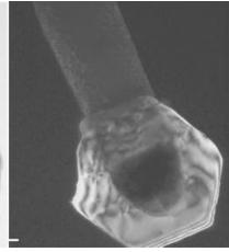
etch in dilute ammonium hydroxide carried out prior to galvanostatic electrodeposition in a pure Cu sulphate aqueous electrolyte at 20-60°C.
