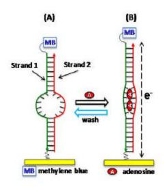
magnitude greater than that in solution measured through gel electrophoresis. The ready reversibility of such an immobilized device on gold surface ensures its re-usability as a biosensor, and offers the potential as a ligand-gated switch in nano-electronics.
