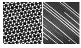
However, no similar templating effect has been reported for the growth of nanostructures on Si(001). We use a dysprosium induced Si(001)  $2\times7$  surface reconstruction to narrow the width distribution of Dy silicide nanowires. These results represent part of the development of nanowire growth techniques towards their eventual application in nanometer scale devices.
